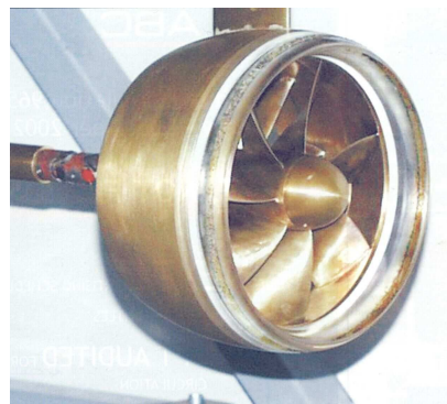
Fig. 3.10 Tip-driven (rim-driven) electric motor propeller (AEG-Jastram and GD prototypes)
