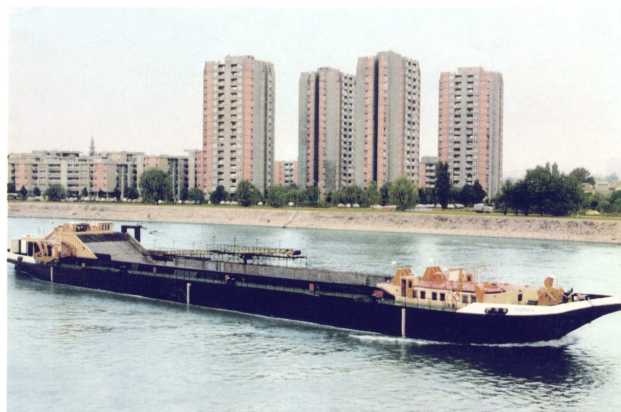
Fig. 4.9 Selfpropelled, self-discharge river bulkcarrier
